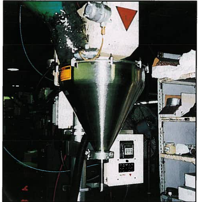
Auger filling machine stores toner prior to filling cartridges
