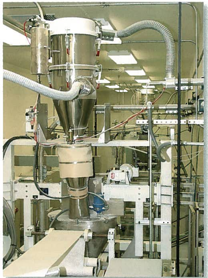
Contract packager/converter Pacon Mfg. fills facial powders using auger fillers. Care must be taken, as the powders often have self-lathering properties.
