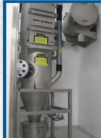
VAC-U-MAX Central Vacuum with Chemical Suppression HEPA2
