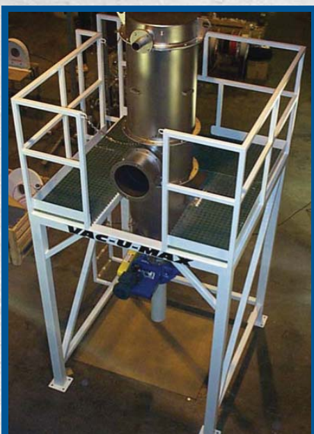
VAC-U-MAX Central Vacuum System with Explosion-Proof Venting
