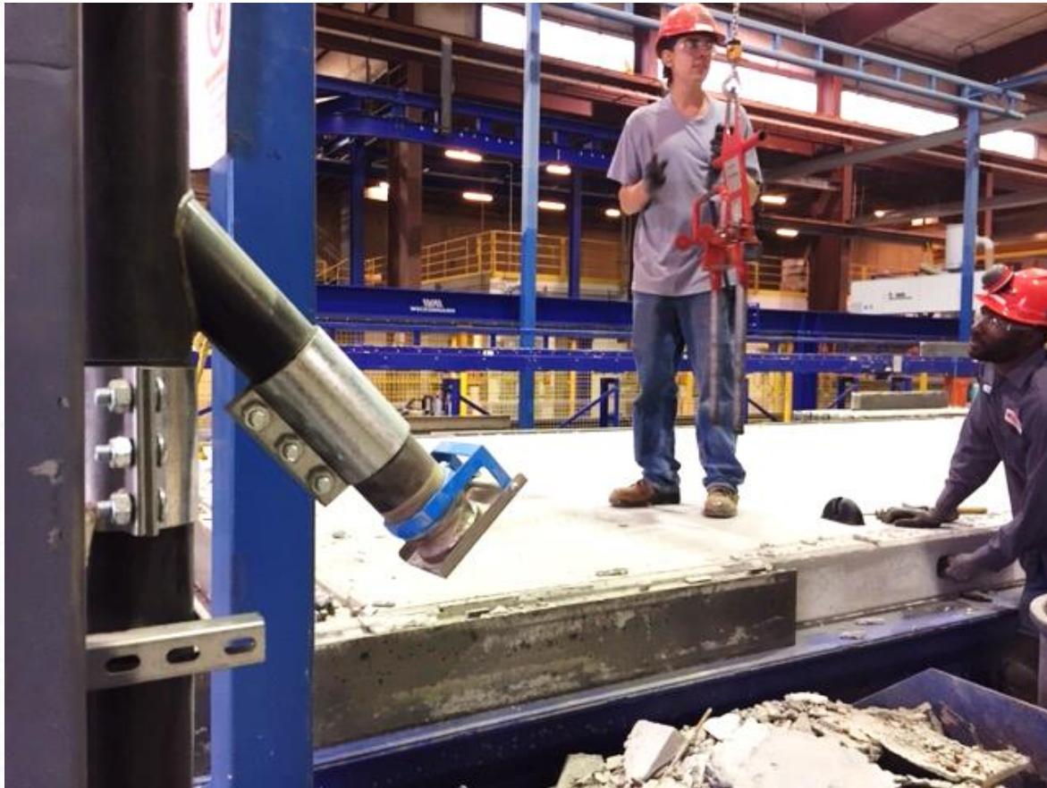
VAC-U-MAX SNAP-CAM inlet valve with spring-loaded cover in form demolding department. Pipe network is sch. 40 steel.
