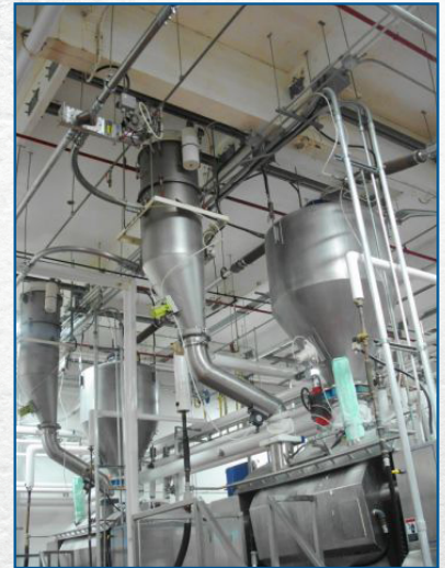
VAC-U-MAX Vacuum Conveying System pneumatically conveying food ingredients to processing line. Material is contained within the system minimizing plant and personnel exposure to dusts and combustible dusts, eliminates manual refill of process equipment - maximizes safety & production.
